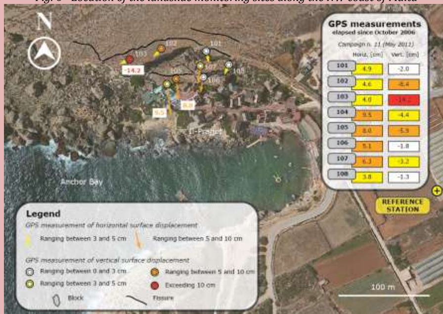
Fig. 7 - Displacements measured at the monitoring site of Anchor Bay, NW coast of Malta
