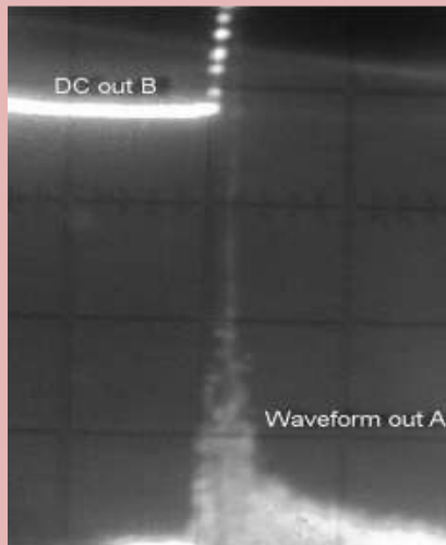
A two-ray oscillogramm, where the acoustic burst arriving on the background of the ambient noise is visible as well as peak value of the signal from the output of the datalogger (clipped).
