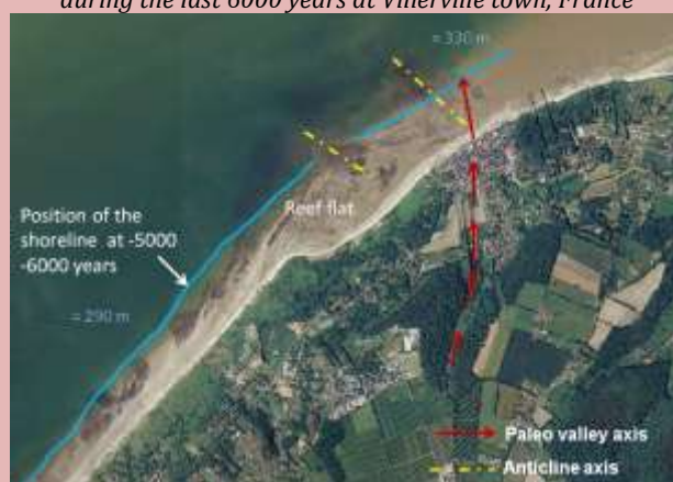
Figure 7: Position of the shoreline at 5000-6000 years BP in front of the Villerville-Cricquebeouf slope, France. The progressive sea erosion during the last 6000 years reach a value of 300 m: the rate of erosion is approx. 5 cm per year for this sea level. But for the future, we have to take into account the relative sea level evolution. On the base of monthly and annual mean sea level measured between 1950 to 2011 at the Dieppe harbor and Le Havre harbor located close to the study sites, the rate of Sea Level Rise (SLR) is respectively 0.53mm per year and 0.18 mm per year since 1960's (Figure 8).
